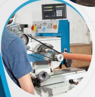
Once covered with rubber mixture, cylinders are put into pressure ovens (autoclave). The cylinders need to wait for at least 48 hours after removal from oven. At the final stage, surface grinding is applied. For this, digital grinding lathes specially designed for grinding rubber-coated printing cylinders are used. After the finishing grinding, some cylinders are subjected to standing on special machines.
